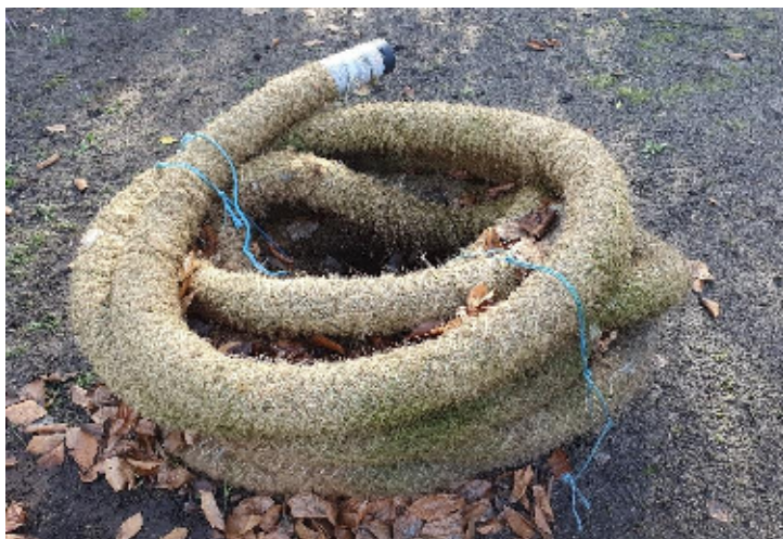
Figure: 27. Traditional drainage hose with coconut fibres
